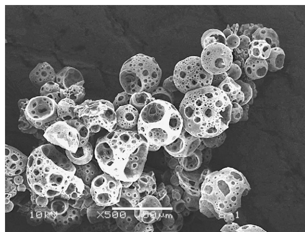
Fig. 10. SEM micrograph of porous blended microspheres of 10/2 (w/w) MPEG- b -PCL/PEG blend (bar = 50 μm).
